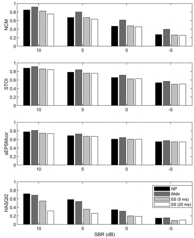
FIG. 2. NCM, STOI, sEPSM<sup>cor</sup>, and HASQI2 values for conditions RNN, SS, and NP for each SBR.
