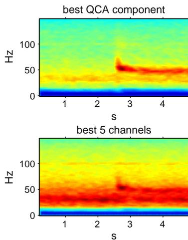
**Fig. 5.** Time-frequency analysis of best QCA component (top) or best 5 sensors (bottom) in the gamma band. Based on short-term Fourier analysis with a 256-point (0.43 s) Hanning analysis window and a 16-point (0.027 s) frame period. Color represents power raised to the exponent 0.2.
