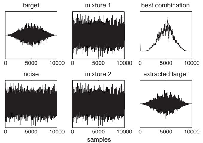
**Fig. 1.** Simulated data. The target consists of 100 repetitions of gaussian noise amplitude-modulated by a sinusoid (left top: one trial). This target is mixed with gaussian noise interference (left bottom) to form two “sensor signals” (center) with  $\text{SNR} = 10^{-8}$ . The algorithm extracts the most reproducible linear combination of cross-products (right top), and uses that to derive a linear combination of “sensors” similar to the target (right bottom).
