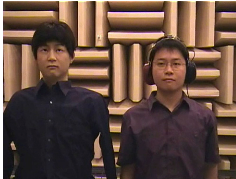
Movie S1. The Telehead dummy head was located in an anechoic chamber. The head position of listeners was measured by a 3D head tracker placed on the top of the headphones. Their head motion was tracked in real-time and sent to the Telehead robotic system (in the actual experiment, the listener was located in a different room, see Fig. 1A for details).
